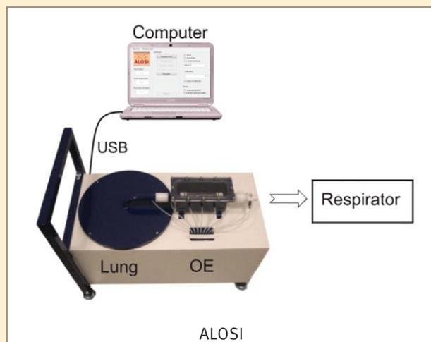
The interface of the lung simulator with the obstructive element (OE) is done via USB and a DA/AD-converter. The respirator that has to be checked must be connected to the lung model.
